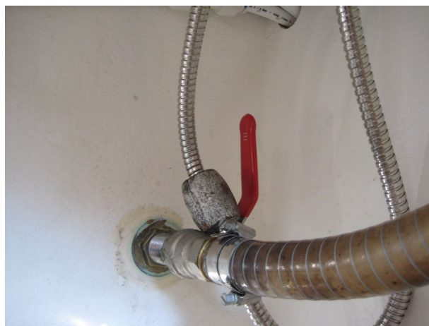
FIGURE 36 – BALL VALVE FITTED TO THROUGH-HULL FOR HEAD SINK DISCHARGE
