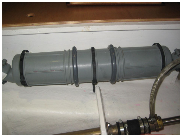
FIGURE 21 – WATERLOCK EXHAUST MUFFLER
