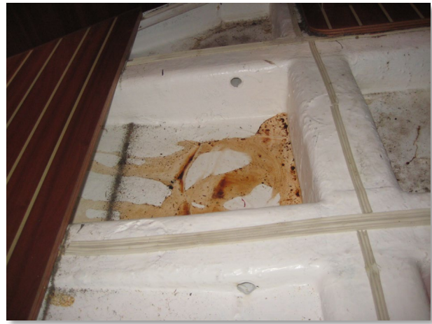
FIGURE 12 – HULL FRAMING BELOW CABIN SOLE
