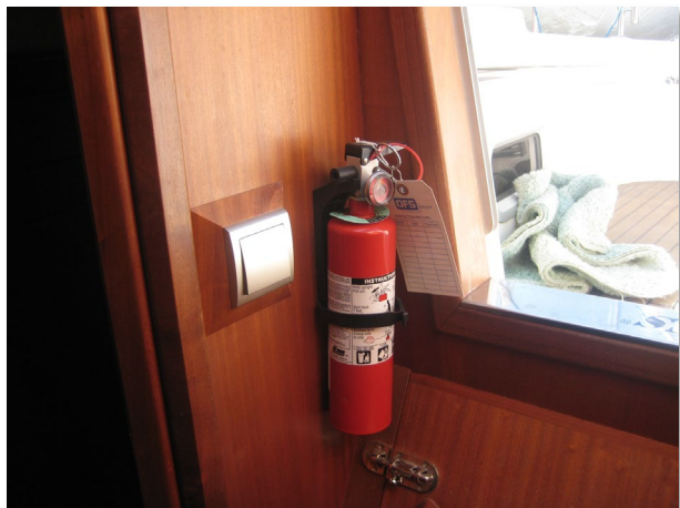
FIGURE 49 – PORTABLE FIRE EXTINGUISHER AT COMPANIONWAY
