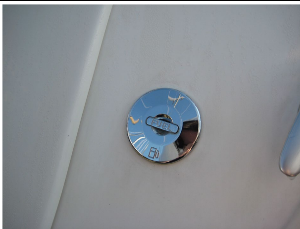
FIGURE 26 – DECK FILL FITTING AT TRANSOM
