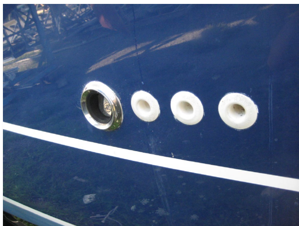
FIGURE 35 – PORT TOPSIDE THROUGH-HULL FITTINGS
