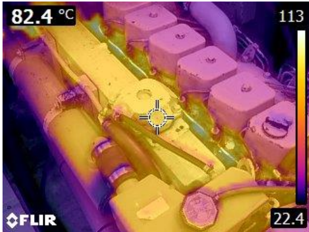
FIGURE 15 - THERMAL IMAGE OF PORT MAIN ENGINE
