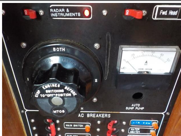
FIGURE 25 – MAIN BATTERY DISCONNECT IN SALON DC PANEL BOARD FIGURE 26 – 8D BATTERY IN ENGINE SPACE
