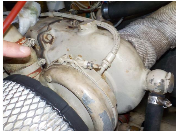
FIGURE 47 - WEEPING FUEL PUMP FITTING AT STARBOARD MAIN ENGINE FIGURE 48 - UNJACKETED TURBOCHARGERS IN ENGINE SPACE
