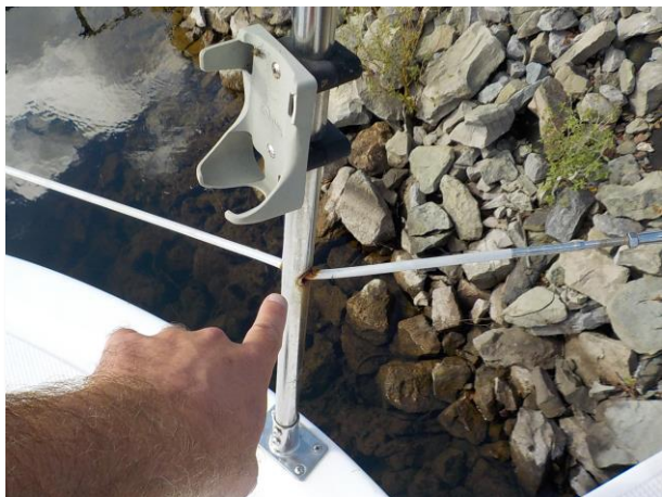
FIGURE 49 – LIFELINE CORROSION AT THE BOW RAIL
