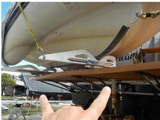
FIGURE 41 – DISTORTION OF AFT PLATFORM
