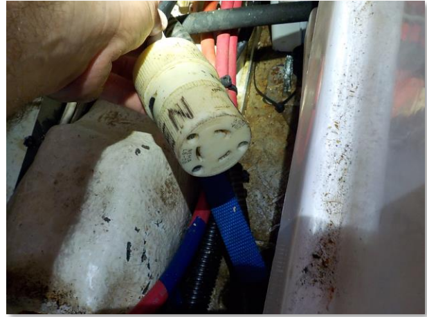
FIGURE 45 - NO SEACOCK ON SANITATION SYSTEM OVERBOARD DISCHARGE FIGURE 46 - EXTENSION CORD LAYING IN BILGE
