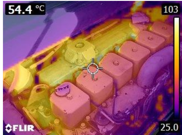
FIGURE 16 - THERMAL IMAGE OF STARBOARD MAIN ENGINE
