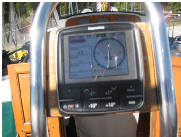
FIGURE 48 – AUTOPILOT CONTROL AT HELM
