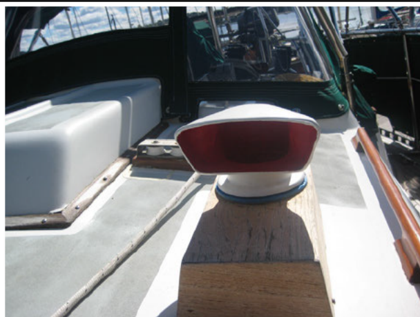
FIGURE 44 – COWL VENT ON CABIN TRUNK
