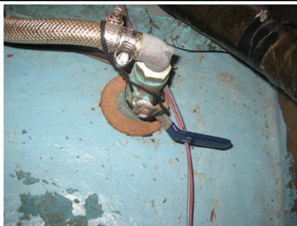
FIGURE 34 – SEA COCK FITTED TO THROUGH-HULL
