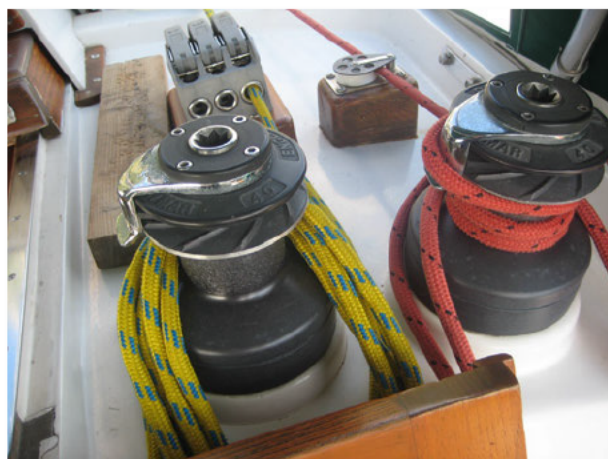
FIGURE 18 – WINCHES FITTED TO STARBOARD SIDE OF CABIN TRUNK
