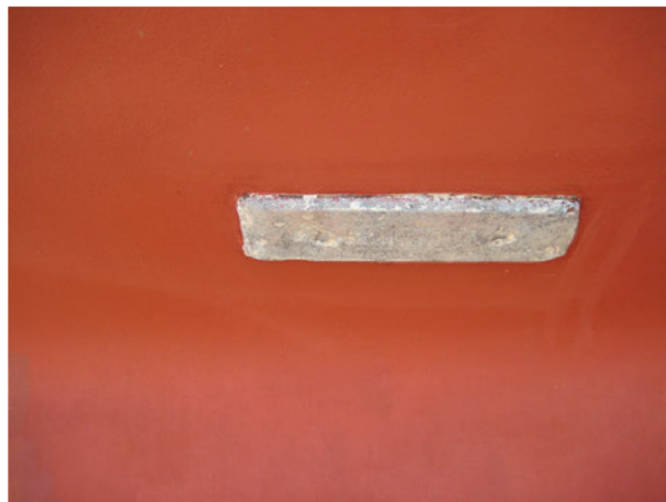
FIGURE 46 - PLATE ANODE ON HULL
