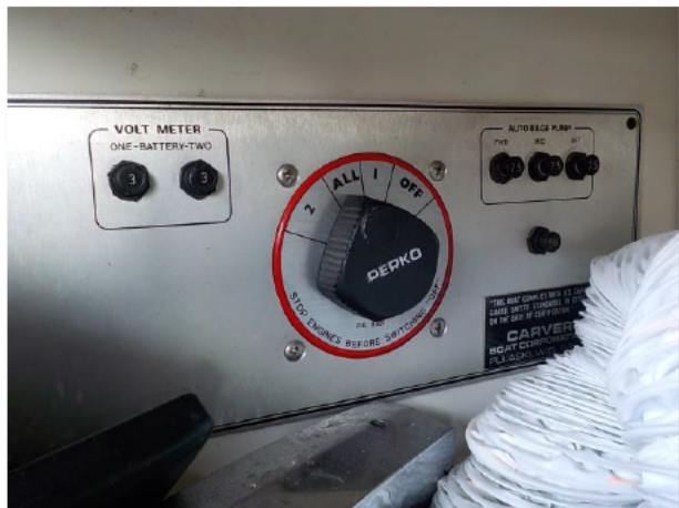
FIGURE 23 - BATTERY MASTER SWITCH IN AFT DECK LOCKER
