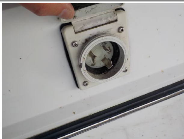
FIGURE 25 - SHORE POWER INLET RECEPTACLE AT TRANSOM
