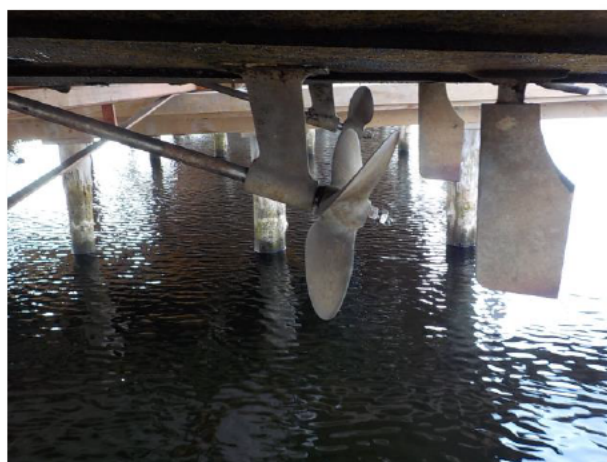
FIGURE 16 - SHAFTS, PROPELLERS AND RUDDERS
