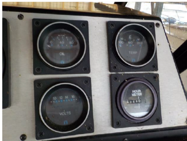
FIGURE 18 – ENGINE GAUGES AT HELM
